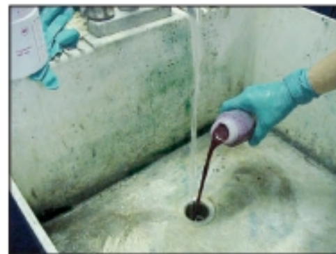
Figure 63: Dye Testing Plumbing (NEIWPCC, 2003)
